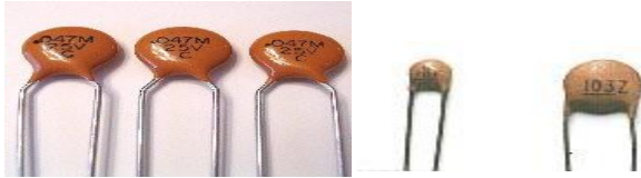
Disc type ceramic capacitor
